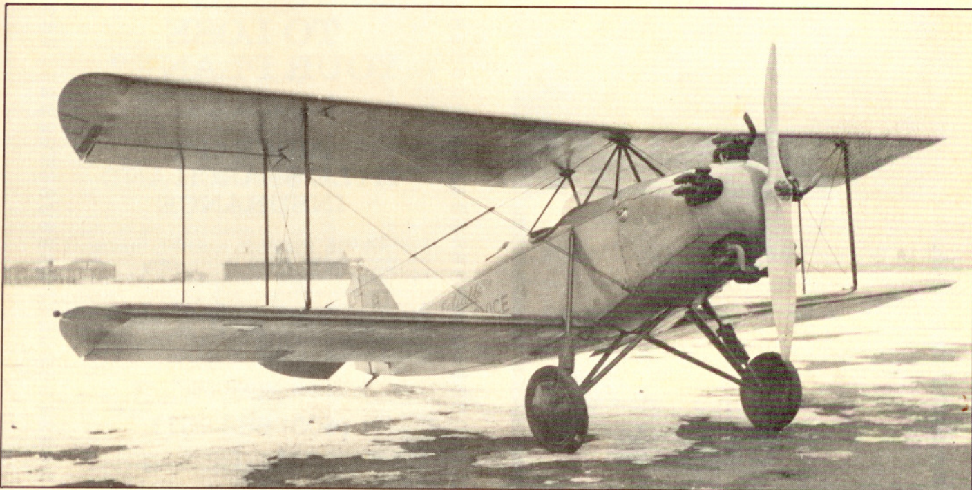
A Bourdon Kitty Hawk B-2 with a 90-hp Kinner K-5 engine. The photo shows the high-pressure wheels also used on the earlier Siemens-powered B-2. Note the rubber-disc shock absorbers.
